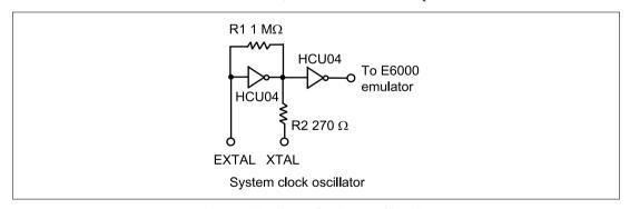
Figure 10 Clock Oscillator Circuits
